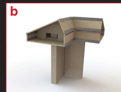
A patented, box eaves beam forms both the soffit and perimeter ceiling
